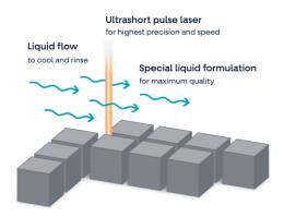
There is a very large potential for Lidrotec in the semiconductor market. When cutting silicon wafers, both a **higher edge quality** and thus better resistance are achieved, as well as **narrower cutting widths** in combination with a reduced crack-stop, so that more chips can be placed on each wafer.
